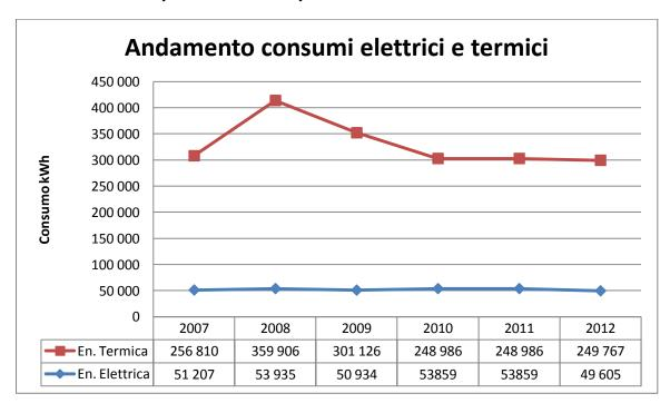
ASP Casa di riposo della Misericordia had high thermal power consumption in 2007, so general board decide to reduce energy cost with some measure. The RCHEP invested in energy saving, with new solar thermal panel in 2009. They retrofit the roof in 2010, but postpone the insulation of attic for next year to have financial capabilities to invest.
